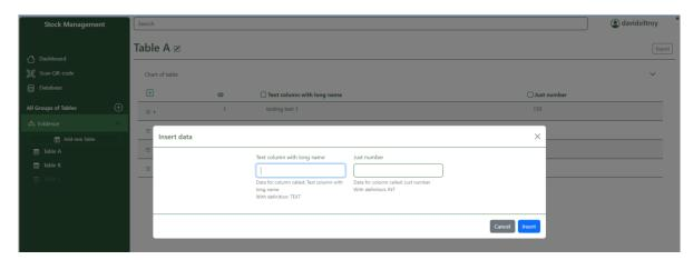
When the table has a column that save foreign keys, then a select input is displayed, giving the different options and saving in the form the ID of the row related to the option selected.
